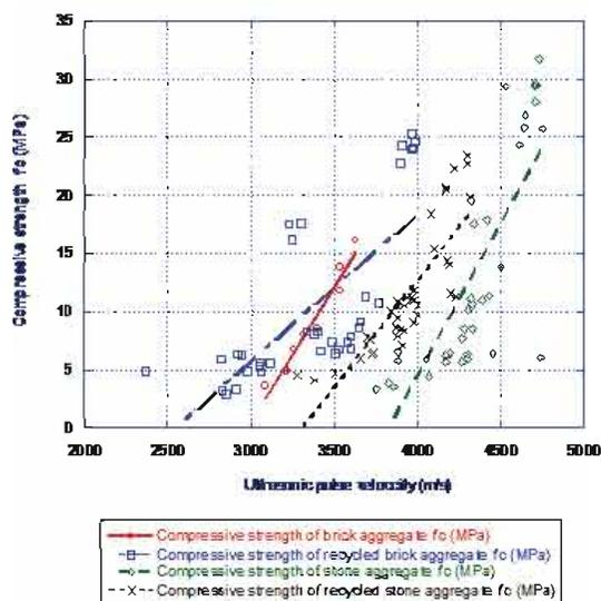
Fig 1: Compressive strength vs. ultrasonic pulse velocity (Coarse aggregate effect)
