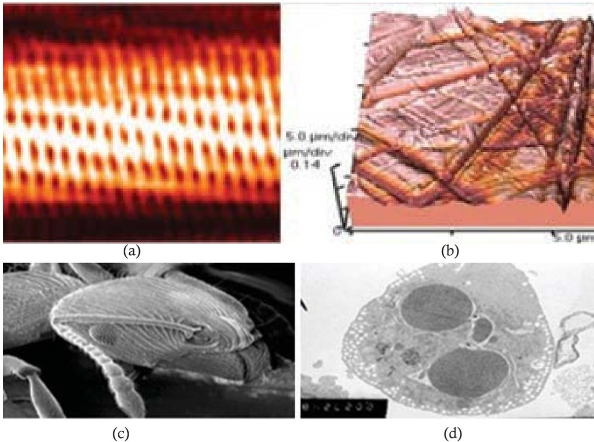
**Fig 5:** (a) STM image (b) AFM Image (c) SEM Image (d) TEM Image (Source: free Wikipedia)
