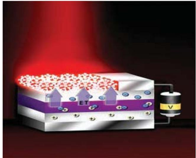
**Fig 4:** This device transfers energy from nano-thin layers of quantum wells to nanocrystals above them, causing the nanocrystals to emit visible light (Source: free Wikipedia)
