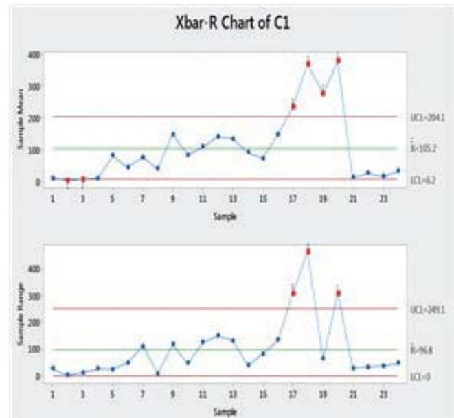
**Fig 2:** Xbar-R chart for the Yarn wastage from outside in Knitting division in DBL
