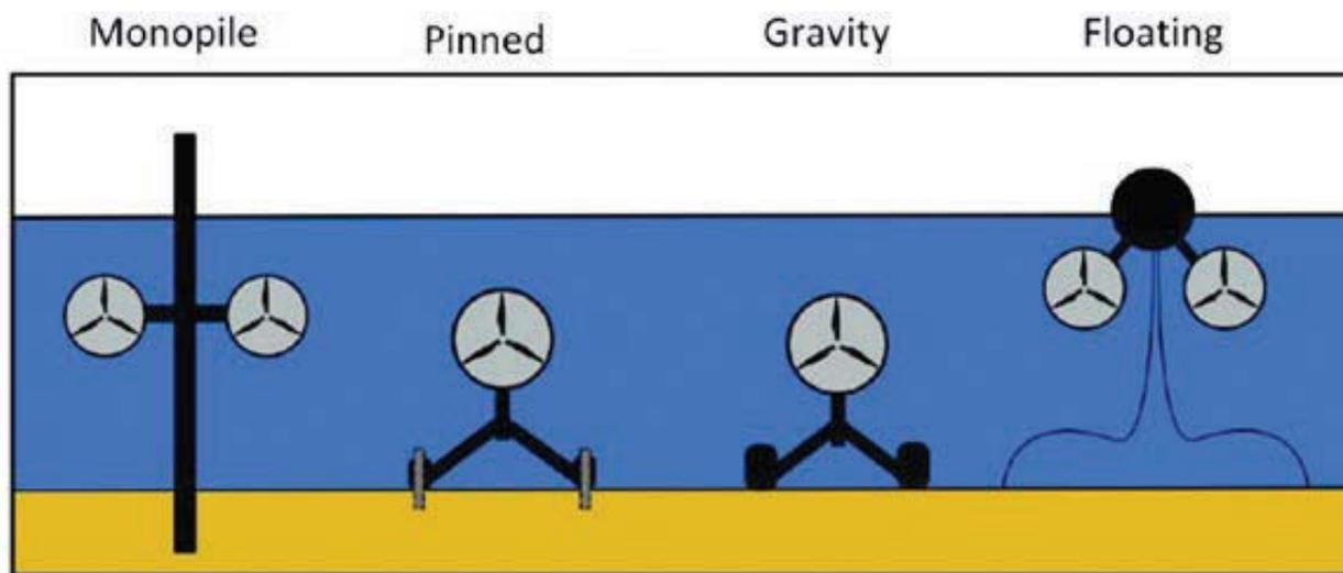
Fig 2. Types of foundation generally used for tidal energy converter.
