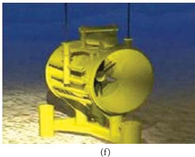
**Fig 1.** Different types of available turbine technologies (a) Vertical axis turbine, (b) Horizontal axis turbine, (c) Oscillating hydrofoil turbine, (d) Tidal kite, (e) Helical screws, and (f) Enclosed tip.
