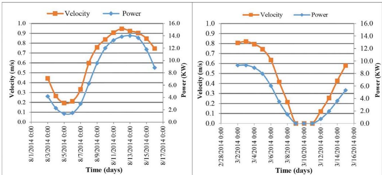
**Fig 5.** Variation of daily average velocity and estimated power covering a Spring-Neap tidal cycle during (a) monsoon period and (b) dry period, for the year 2014.
