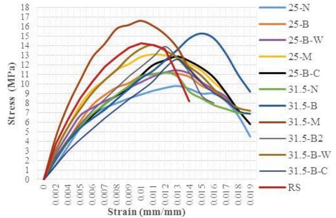
**Fig 4.** Stress vs. Strain for different Column samples
