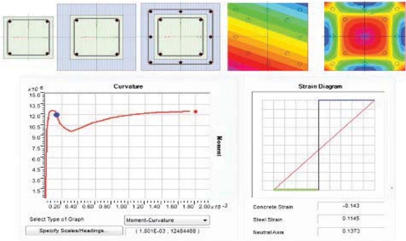
Fig 6. Jacket section in ETABS2015 and Sap2000 with moment curvature and typical strain diagram.
