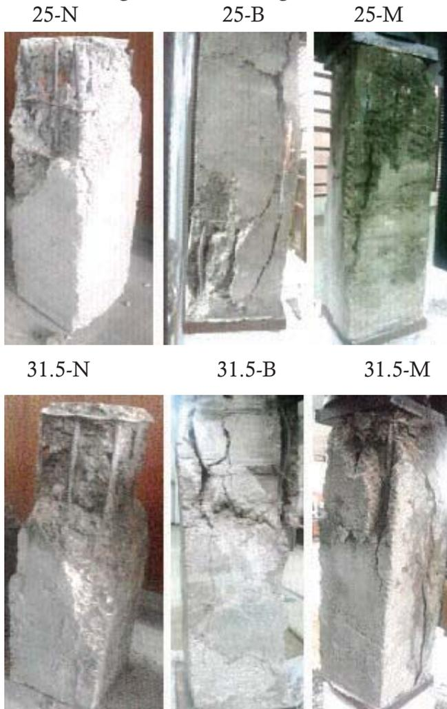
**Fig 3.** Typical failure pattern of sample with their designation below
