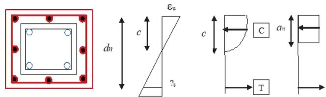
Retrofitted Column Strain Diagram Tension Compression  $T + T_{eff} = T_{eff}$
