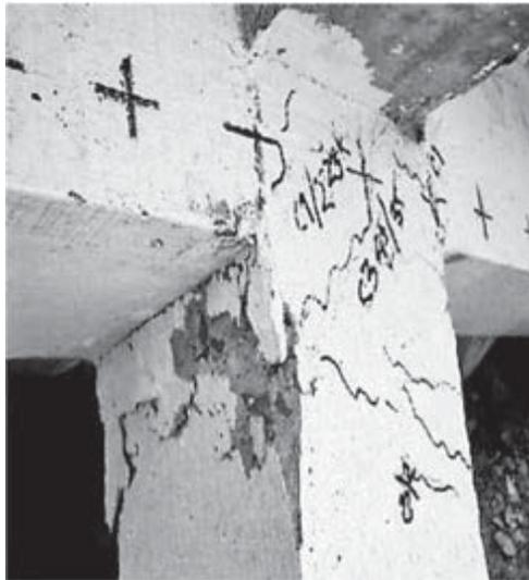
**Fig 28. Joint Failure of Model 1**
