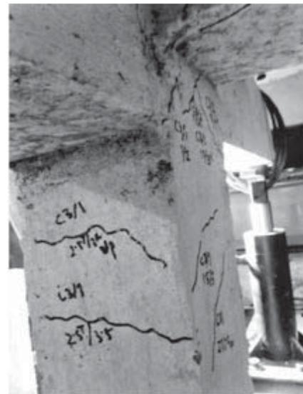
Fig 23. Column Failure, Model 2
