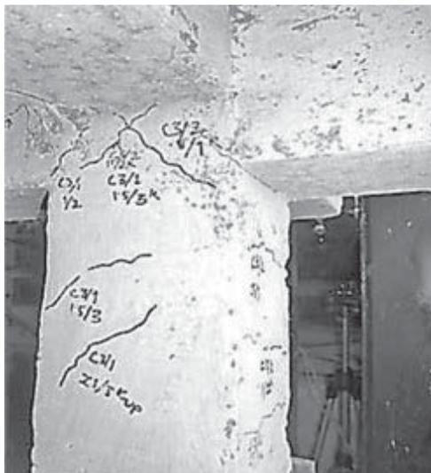
**Fig 29. Joint Failure of Model 2**
