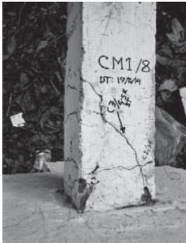
Fig 21. Upper Column Failure, Model 1
