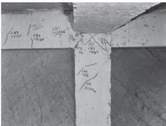
Fig 16. Model 2 Beam Cracks
