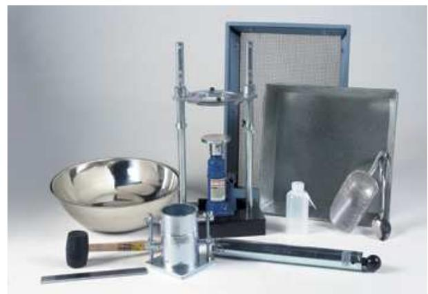
Figure 4.2: Standard proctor test apparatus (geotech.org)
