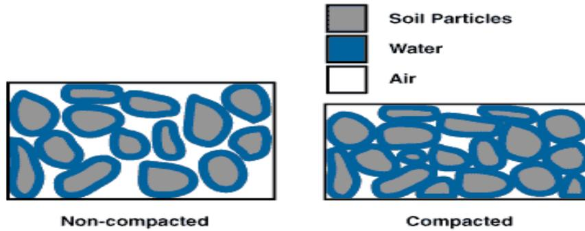
Figure 2.1: Effects of compaction on pore space
