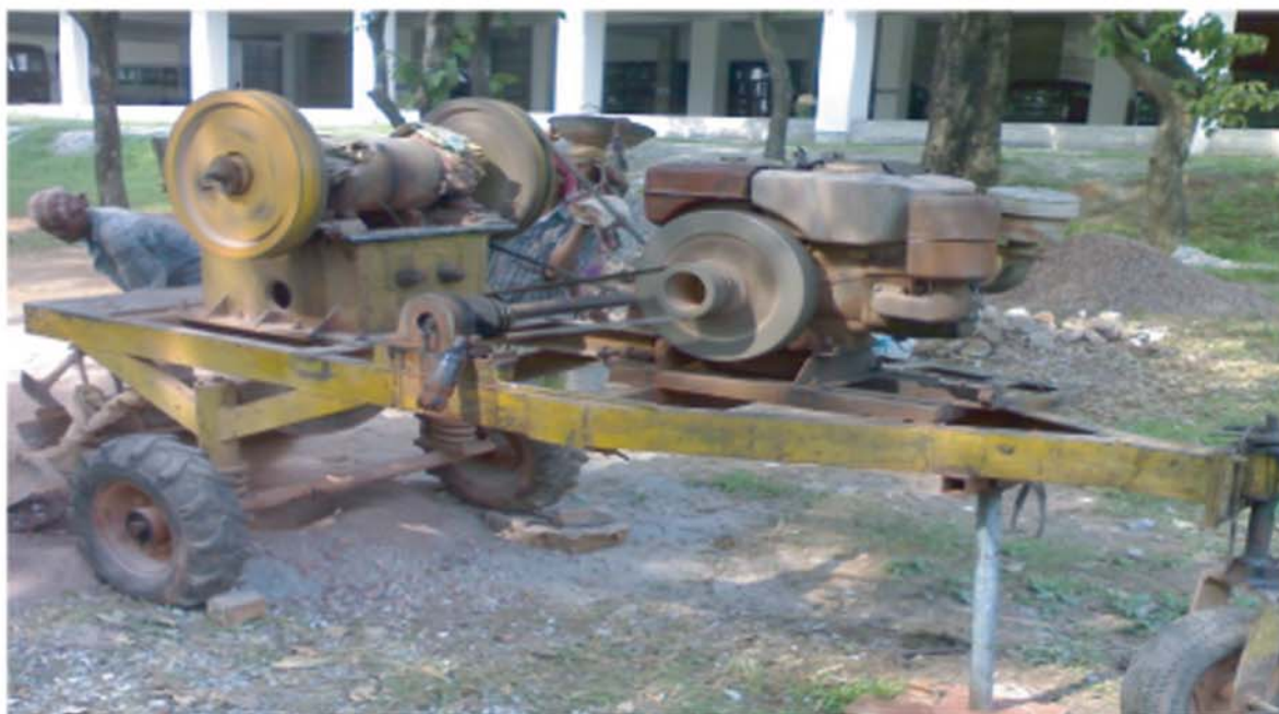
Figure 1: Locally available stone and brick crushing machine in Bangladesh
