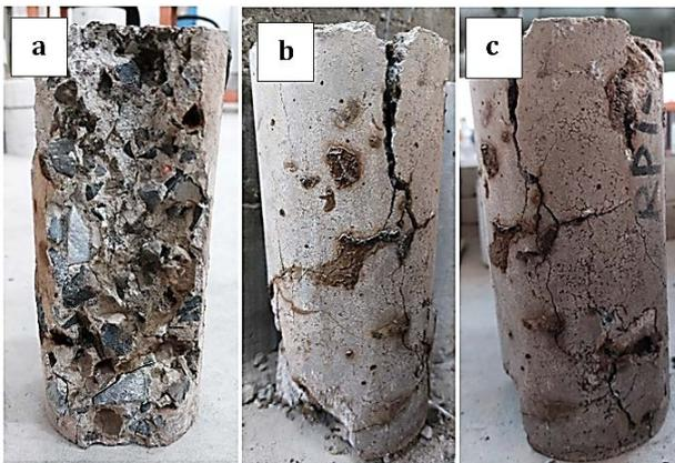
**Figure 3:** Concrete failures at  $800^{\circ}\text{C}$  (a) NC, (b) GRA (35%), and (c) CRA (35%)
