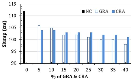
Figure 4: Slump value of varying concrete mixtures
