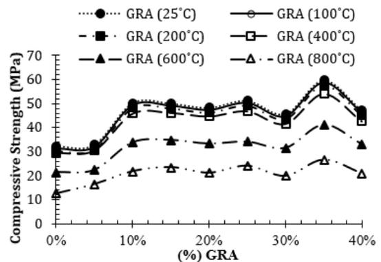
Figure 6: Compressive strength at different temperatures (GRA)
