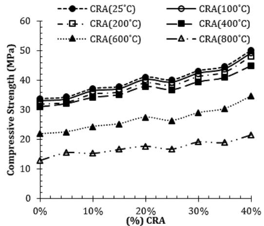
Figure 5: Compressive strength at different temperatures (CRA)
