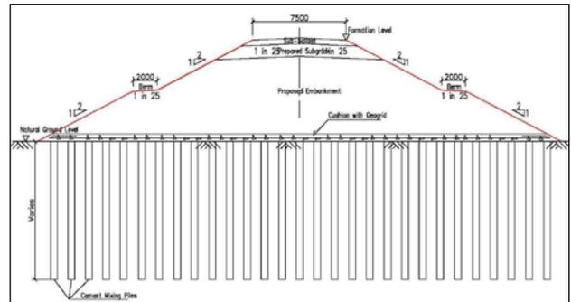
**Figure 8:** Cross section of embankment with Cement Mixing Piles.
