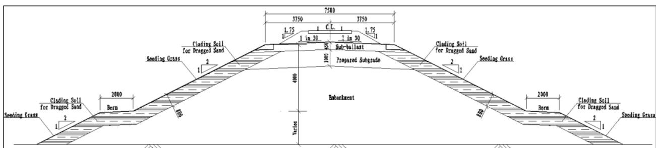
Figure 5: Typical cross section of embankment with height  $\geq 4.0\text{ m}$
