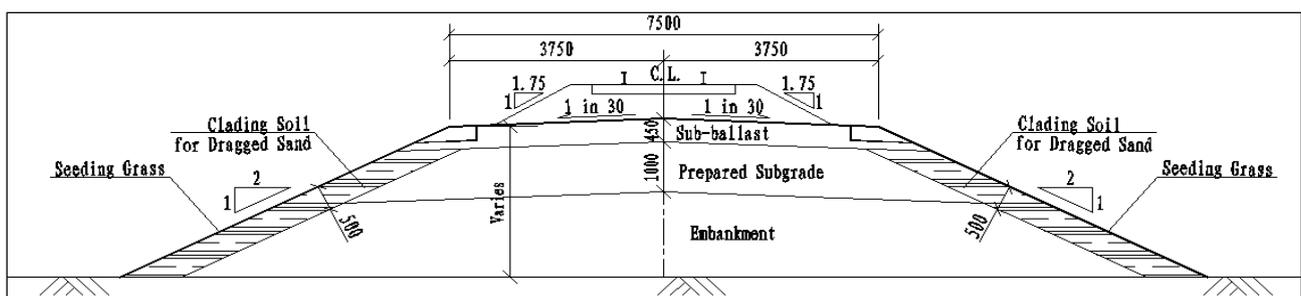
Figure 4: Typical cross section of embankment with height  $\leq 4.0\text{ m}$
