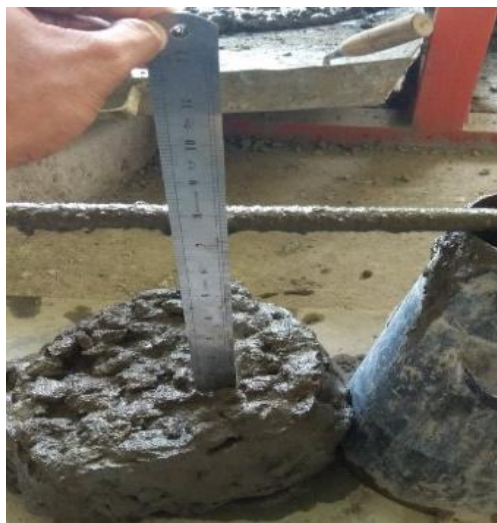
Figure 4: Slump test of concrete with w/c ratio of 0.4
