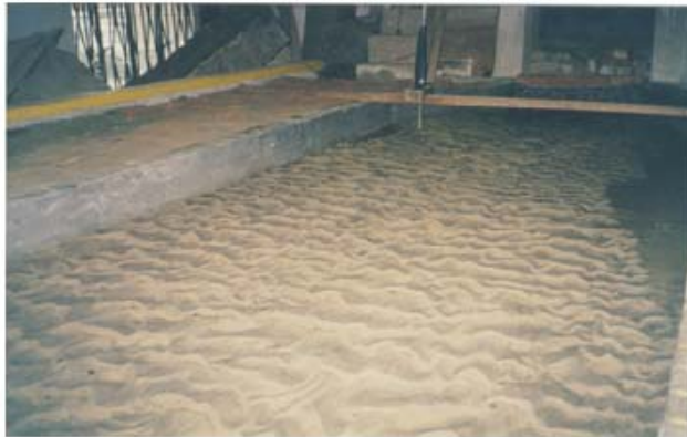
Fig 7. Ripple formation and Ripple Height Measurement
