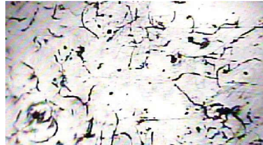
Figure-6: Microstructure of Bangladeshi Cylinder Liner (x400)
