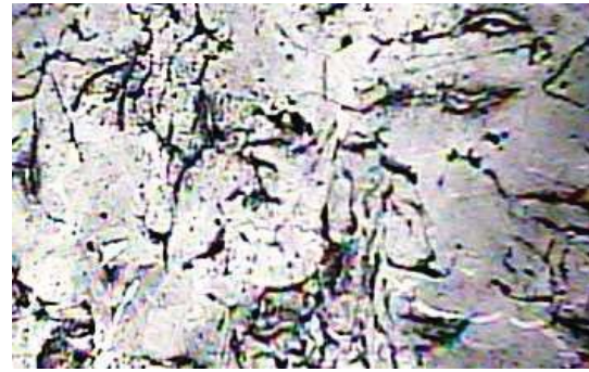
Figure-5: Microstructure of Chinese Cylinder Liner (x400)
