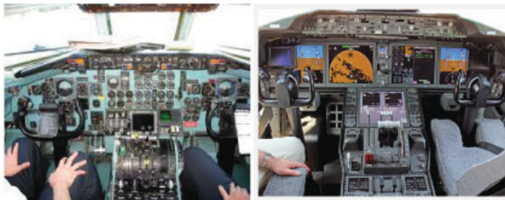
Fig-2: Photographs comparing a 1979, DC-80 Cockpit (left) & 2012, Boeing-787 All-Glass-Cockpit, (right) Pictures: (L) http://aluwings.blogspot.com ; (R) http://airpigz.com/blog
