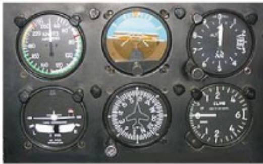
Fig 1: Basic-6 group of Instruments. From top left clockwise: ASI, Artificial Horizon, Altimeter, VSI, Directional Gyro & TSI.
