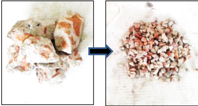
Figure 1: Demolished brick concrete block and recycled brick aggregates
