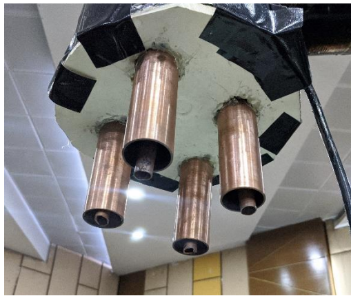
Figure 6: Picture showing spaces inside copper tubes for charge injection
